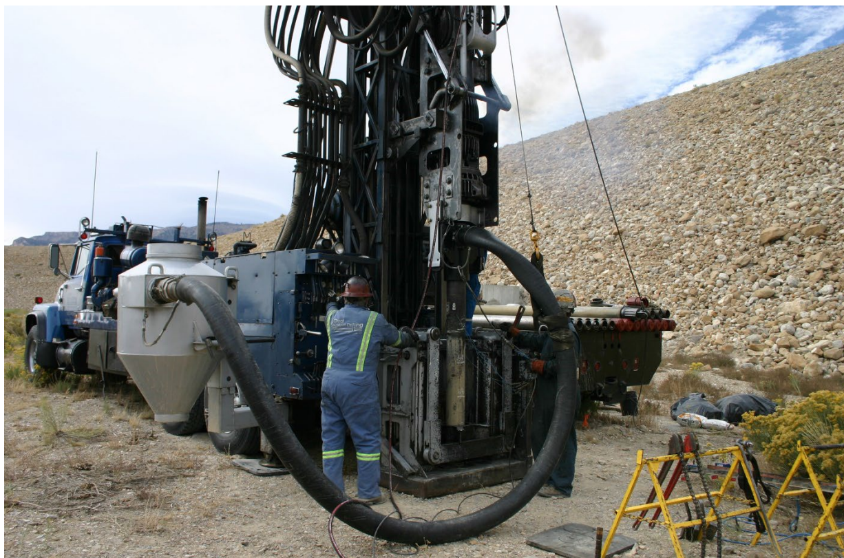
Figure 46. Energy measurements being acquired on the drill string during Becker Penetration Testing.
