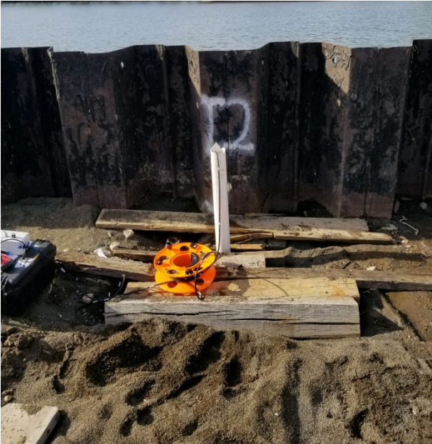
Figure 54. LITE probe in PVC borehole.
