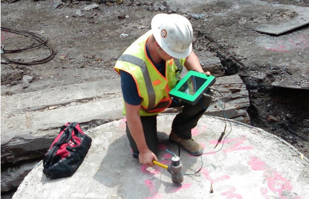
Figure 25. Low strain pile integrity test
