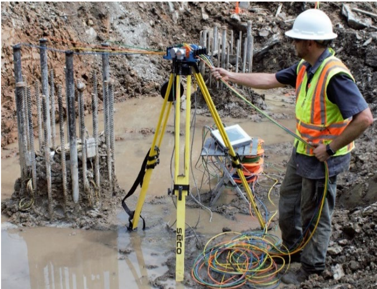
Figure 18. Typical field set-up of multiple transceiver CSL test.
