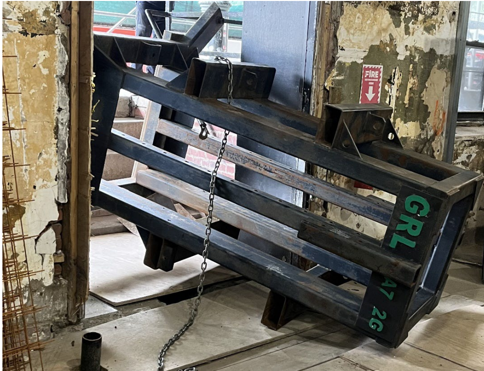
Figure 6. The modified dynamic load testing frame.
